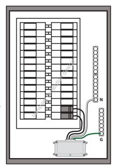
Note: Check local electrical codes before installing SPD inside panel. Consider ordering TPX-RemoteLightKit for remote status indicator (fiber cable & lens plate) for inside panel installations.
